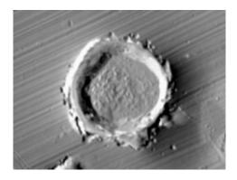
A scanning electron image of one of the iron metal grains analysed.
