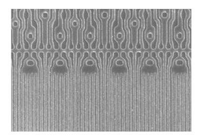
In this scanning electron microscope image, the complex pattern was transferred using rigiflex lithography, a whole device printing method that can easily fabricate large, multi-color displays using a step and repeat process. The lines are 270 nanometers wide and the space between the lines is 80 nanometers. Photo credit: Choi et al.
