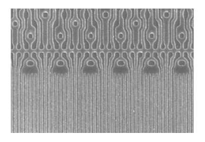
In this scanning electron microscope image, the complex pattern was transferred using rigiflex lithography, a whole device printing method that can easily fabricate large, multi-color displays using a step and repeat process. The lines are 270 nanometers wide and the space between the lines is 80 nanometers. Photo credit: Choi et al.
