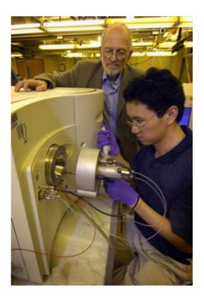
R. Graham Cooks, at left, Purdue&acutes Henry Bohn Hass Distinguished Professor of Analytical Chemistry, watches as doctoral student Hao Chen places a sample into a heating device as part of a new procedure called atmosphericpressure thermal desorption ionization. (Purdue University photo/David Umberger)
