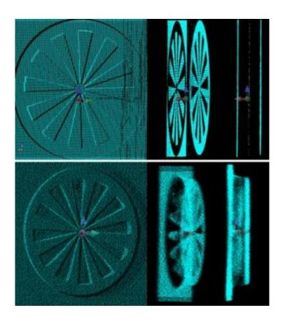
The two sets of images above show data obtained from two instruments used to measure a slotted disk. The top set shows less noisy or more precise data. Credit: NIST
