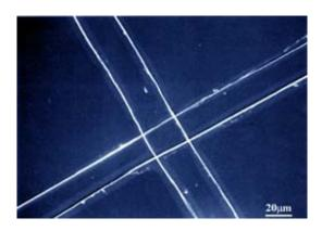
These orderly rows of nanofibers were created using the new near-field electrospinning process. Until now, electrospinning produced random tangles of fibers.
