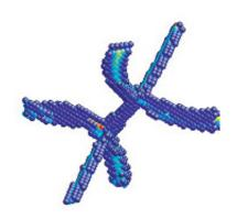
Atomistic simulation reveals the multijunctions in the metal molybdenum.
