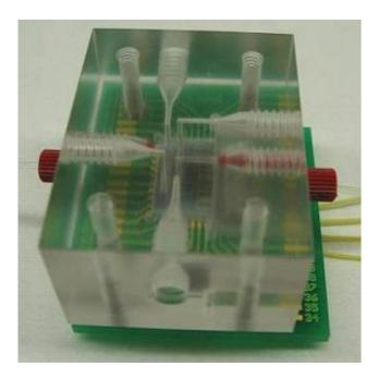
The lab-on-a-chip is a miniaturized, portable version of a blood-count machine. On long missions, astronauts will need the ability to analyze blood samples in realtime to diagnose infection, allergies, anemia or deficiencies in the immune system. Credit: Photo courtesy of Y. Tai, California Institute of Technology
