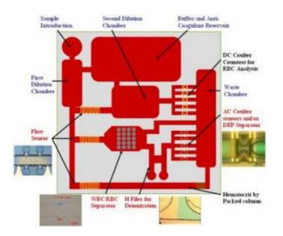
Dr. Tai and his collaborators designed micro-sized valves, pumps and flow chambers that operate and fit together in the lab-on-a-chip. The tiny device requires less than a drop of blood in order to identify components such as red and white blood cells, lipids, proteins or oxygen molecules. Credit: Image courtesy of Y. Tai, California Institute of Technology.
