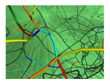
A computer graphic shows defect lines in a crystal. In the foreground, four different types of lines join together to form a "multi-junction," a previously unrecognized microstructure imparting strength to materials
