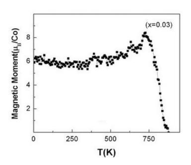
Magnetization as a function of temperature for epitaxial  $Ce_{0.97}Co_{0.03}O_{2-d}$  film grown on LaAlO<sub>3</sub>(001) substrate. Credit: NMRL, University of Utah, [A. Tiwari et al., Applied Physics Letters 88, 142511-1, 2006]
