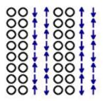
A schematic diagram illustrating stripe order in materials such as LBCO 1:8. Circles indicate the hole-doped copper sites. Up and down arrows represent magnetic moments (orientation of electron spins) on undoped copper sites. Alternating "stripes" of holes and magnetic regions may be necessary for superconductivity.
