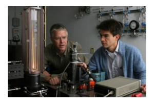
Sandia National Laboratories researchers Chris Shaddix (left) and Alejandro Molina discuss an experiment to determine the best proportion of oxygen and carbon dioxide for oxy-combustion of coal. (Photo by Bud Pelletier)
