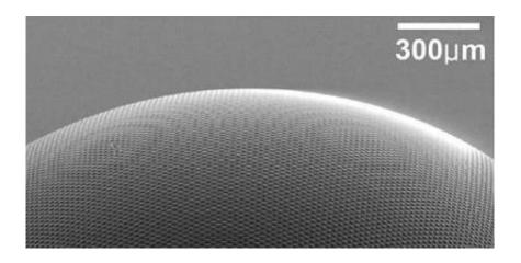
A scanning electron microscope image of the surface of an artificial compound eye shows some of the 8,700 hexagonal microlenses that make up its surface. (Luke Lee photo, courtesy of Science magazine)
