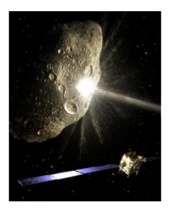
The Impact moment on the Don Quijote mission: The Orbiter spacecraft (Sancho) has retreated to a safe distance to observe how the Impactor spacecraft (Hidalgo) crashes into the asteroid. After the Impact Sancho will come closer and inspect the changes. Credits: ESA - AOES Medialab
