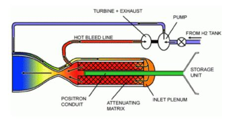
A diagram of a rocket powered by a positron reactor. Positrons are directed from the storage unit to the attenuating matrix, where they interact with the material and release heat. Liquid hydrogen (H2) circulates through the attenuating matrix and picks up the heat. The hydrogen then flows to the nozzle exit (bell-shaped area in yellow and blue), where it expands into space, producing thrust. Credit: Positronics Research, LLC
