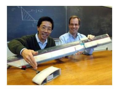
Professors Yet-Ming Chiang, left, and Steven Hall show components of their electrochemically actuated morphing rotor prototype (foreground) as well as a reduced-scale model (background) of a previous technology that uses piezoelectrics as the active materials. Photo / Donna Coveney
