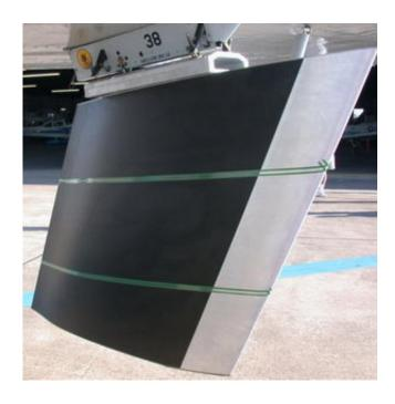
A close-up of the experimental airfoil mounted under the wing of the Aggies&acute plane.
