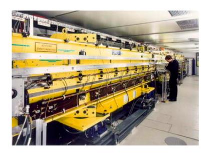
Building the free-electron laser. This so called undulator is an arrangement consisting of many magnets. It is used to produce laser light with short wavelenghts. Source: DESY
