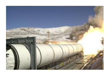
A two-minute static firing of a space shuttle technical evaluation motor was successfully completed March 9 at ATK Thiokol, a unit of Alliant Techsystems, Inc., in Promontory, Utah, north of Salt Lake City. The test included 26 specific objectives and used 89 instrumentation channels to collect and evaluate motor performance. Results will be published in a final report later this year. (ATK Thiokol)
