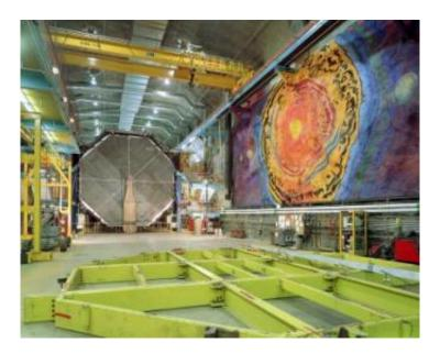
The Main Injector Neutrino Oscillation Search (MINOS) experiment studies a neutrino beam using two detectors. The MINOS near detector, located at Fermilab, records the composition of the neutrino beam as it leaves the Fermilab site. The MINOS far detector, located in Minnesota, half a mile underground, again analyzes the neutrino beam. This allows scientists to directly study the oscillation of muon neutrinos into electron neutrinos or tau neutrinos under laboratory conditions.
