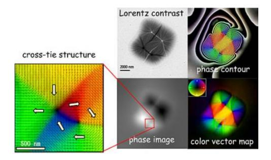
An individual magnetic element showing local magnetization under an applied field via magnetic phase imaging and reconstruction methods.
