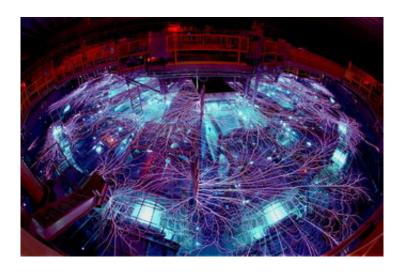
Sandia&acutes Z machine firing. The "arcs and sparks" formed at the water-air interface travel between metal conductors. (Photo by Randy Montoya)
