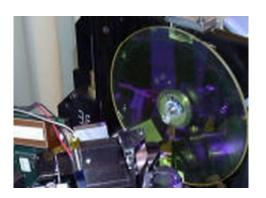
InPhase Technologies announced today that it has demonstrated the highest data density of any commercial technology by recording 515 gigabits of data per square inch. Holographic storage is a revolutionary departure from all existing recording methods because it takes advantage of volumetric efficiencies rather than only recording on the surface of the material. To compare, magnetic disk drives allow 300 gigabits per square inch data density.
