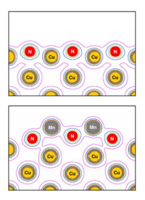
This image shows a calculated cross-section of the CuN surface layer before (top) and after Mn atoms are placed on the surface. (This calculation is not part of the Science Express paper itself; it was done for another paper by colleague Chiung-Yuan Lin.) Credit: IBM
