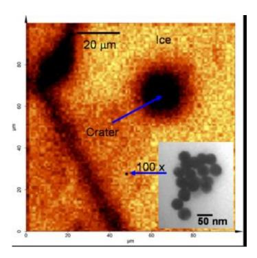
A cluster of gold nanoparticles 50 nanometers in diameter created a much larger crater in the ice sample, shown here. Courtesy of Hugh Richardson
