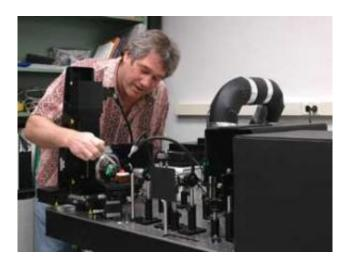
Robert Downs adjusts a piece of the mineral corundum in a Raman spectrometer. Rubies are red-colored corundum; sapphires are blue-colored corundum. Photo courtesy of the Downs laboratory, The University of Arizona.
