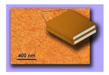
Atomic force microscopy image of aligned nanofibrils of a highly conducting plastic. Each nanofibril is made of stacks of regioregular polythiophene (RRP) molecules. Charge carriers move particularly well along the length of RRP molecules, perpendicular to the rows of nanofibrils. Credit: Image courtesy of Tomasz Kowalewski, Carnegie Mellon University
