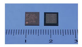
Toshiba Corporation announced the introduction of the world's first MDDI-compliant LCD controller optimized for cell phones equipped with high-resolution VGA LCD displays. Dubbed the MDDI LCD Bridge and designated TC358720XBG, the highly integrated, single-chip device is well suited for the new generation of advanced multimedia cell phones with MDDI interfaces, including 3G cellular handsets.
