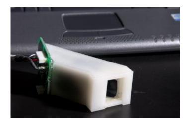
A prototype spectrometer made using Georgia Tech's new technology. This spectrometer can be plugged into a lap top and used for environmental sensing.
