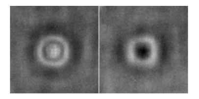
On the left, a microlens is in the 'on' state and ready to detect. The right shows the microlens in the 'off' state after it has detected its target chemical.
