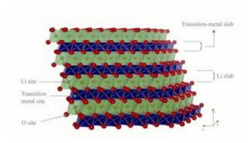
The structure of lithium nickel manganese oxide consists of layers of transition metal (nickel and manganese, blue layer) separated from lithium layers (green) by oxygen (red). Image courtesy / Ceder Laboratory
