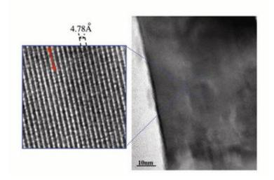
An electron micrograph of lithium nickel manganese oxide. The white layers are composed of nickel manganese oxide, and the dark layers represent lithium. Image courtesy / Ceder Laboratory
