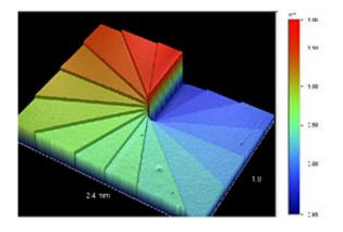
Measured surface profile of the helical vortex mask used in lab experiments. The pitch of the mask corresponds to two full waves of phase delay for green light. This false color image was obtained by Joanna Schmit (Veeco, Inc.) The mask was made by Eric Johnson of the University of Central Florida. (Graphic: Courtesy of Grover Swartzlander)
