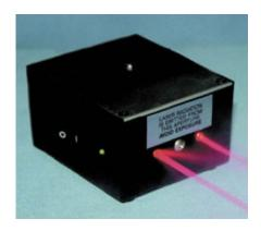
The Laser Scaling Device attaches directly to a camera and projects a pattern of dots into the field of view. This pattern appears in the photograph along with the image of the object under investigation, enabling the viewer to measure the size of the object. Credit: NASA
