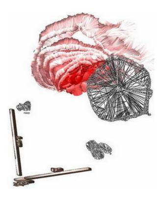
The 3D gradient of the crystallographic orientations in an intermetallic ironaluminium specimen (lattice curvature) close to a very hard Laves phase (appears as a transparent net). The various layers of colour indicate increasing changes in the crystal orientation from the reference point directly at the interface between matrix and Laves phase in two degree misorientation intervals. Image: Max Planck Institute for Iron Research
