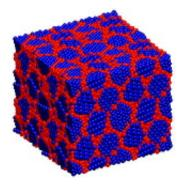
This conceptual drawing shows the structure of a nickel-tungsten alloy that promises a safer alternative to chromium. The nano-sized crystals (blue) are mostly composed of nickel, and are joined together by regions rich in tungsten (red). Photo courtesy / Schuh Lab
