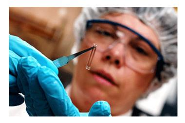
Deborah McGee of CardioMEMS examines an EndoSure sensor in the company's clean room facility in the ATDC Biosciences Center located at Georgia Tech's Environmental Science and Technology Building. The sensor is implanted to measure pressure in an aneurism being treated by a stent graft. Georgia Tech Photo: Gary Meek
