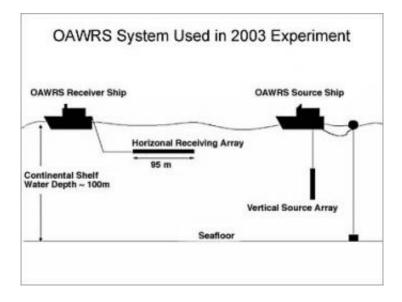
Setup for the remote sensor system used to measure fish populations off Long Island, N.Y., by researchers from MIT, Northeastern University and the Naval Research Laboratory. Image courtesy / Nicholas Makris
