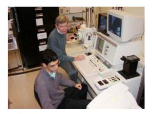
Alireza Nojeh (front) and Fabian Pease use a scanning electron microscope to view carbon nanotubes.
