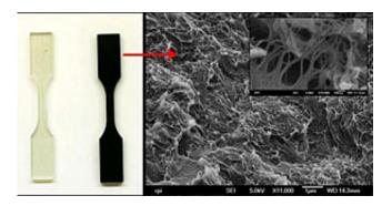
From left to right, an untreated sample of polymer material, the new nanocomposite, and a scanning electron microscopy image showing the nanotubes dispersed in the polymer resin. Credit: Rensselaer/Koratkar
