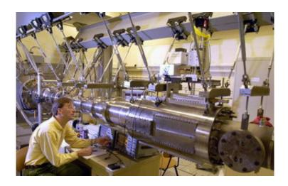
Image: Steven Schneider, an aerospace engineer and professor in Purdue&acutes School of Aeronautics and Astronautics, operates the university&acutes one-of-a-kind wind tunnel, which runs quietly at Mach 6, or six times the speed of sound. (Purdue photo/David Umberger)
