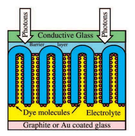
Integration of transparent nanotube array architecture into dye solar cell structure.
