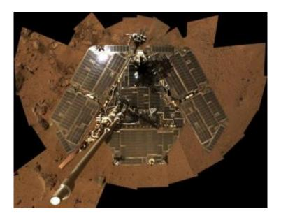
The most recent self-portrait of NASA's Mars Exploration Rover Spirit shows the solar panels still gleaming in the martian sunlight and carrying only a thin veneer of dust two years after the rover landed and began exploring the red planet.
