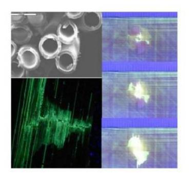
Hollow fibres just 30 micrometres in diameter tread the new material. When damage occurs, the fibres break releasing liquids that seep into the cracks and harden, repairing the damage. Credits: ESA
