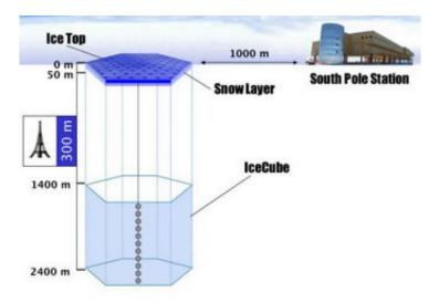
Diagram of IceCube. IceCube will occupy a volume of one cubic kilometer. Here we depict one of the 80 strings of opctical modules (number and size not to scale). IceTop located at the surface, comprises an array of sensors to detect air showers. It will be used to calibrate IceCube and to conduct research on highenergy cosmic rays. Author: Steve Yunck, Credit: NSF
