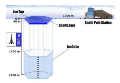
Diagram of IceCube. IceCube will occupy a volume of one cubic kilometer. Here we depict one of the 80 strings of opetical modules (number and size not to scale). IceTop located at the surface, comprises an array of sensors to detect air showers. It will be used to calibrate IceCube and to conduct research on high-energy cosmic rays. Author: Steve Yunck, Credit: NSF
