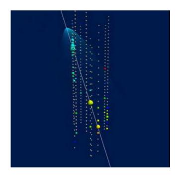
The IceCube telescope and its predecessor, AMANDA, use optical sensors to locate the sources of high energy neutrinos. This picture shows the on-line display of neutrino event recorded by AMANDA. Author: Jodi Lamoureux, Credit: NSF
