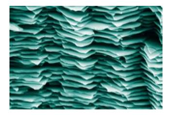
This metal-ceramic composite (top image) developed by the Berkeley Lab team resembles the microstructure of nacre (bottom image). Images courtesy of Tomsia et al.
