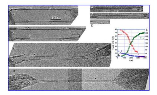
Image updated: A single-walled carbon nanotube of 75 nanometers can stretch to 84 nanometers before it breaks. Image courtesy of Jianyu Huang.
