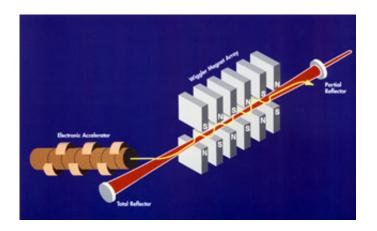
The principle behind the free-electron laser: a beam of accelerated electrons is guided through a series of magnets which, by changing the polarity, "wiggle" the beam at the necessary frequency to produce the desired wavelength. (Vanderbilt University)
