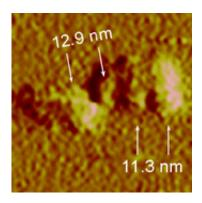
Atomic force microscope image of a protein nanospring reveals its coiled structure.
