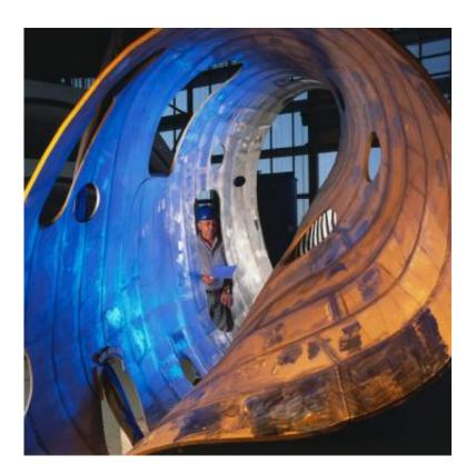
Part of the plasma chamber of Wendelstein 7-X: Twenty of these elements are joined to form a ring shaped in keeping with the twisting contours of the plasma. The ports in the vessel grant access for heating and measuring facilities. (Photo: IPP, W. Filser)
