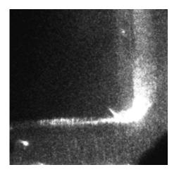
Turning point: A single atomic ion is shuttled back and forth around a corner. Light scattering makes the corner electrode visible.
