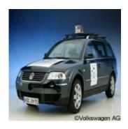
Volkswagen Passat with the sensing platform, driver warning and vehicle control systems.
